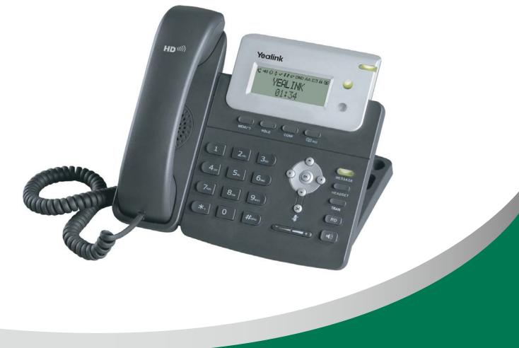
Yealink expands its lineup of IP phones with a new entry-level product SIP-T20P. It is equipped with TI TITAN chipset and 2x15 characters LCD, offers 2 VoIP accounts, high-definition voice, broad range of voice codecs, security protection for privacy, rich features including XML phonebook, headset, PoE, PnP Auto-provision, and seamlessly work with the leading IP-PBX and soft switch.
